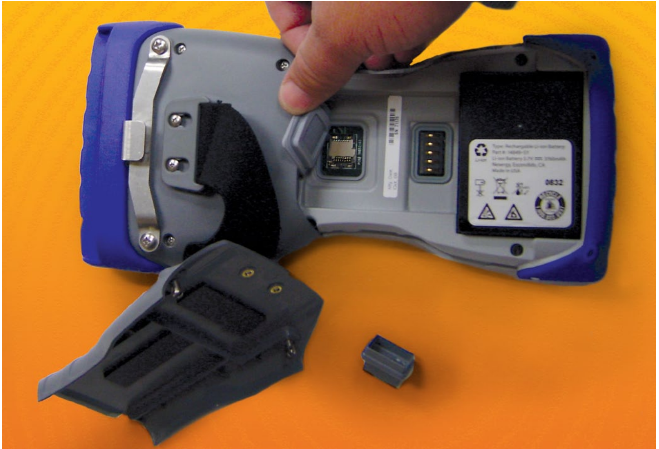
The rear cover reveals space for two removable batteries. Beneath the second battery space is the microSD memory card slot protected by a rubber plug. Also seen here are the tripod hook and the elastic hand strap.
