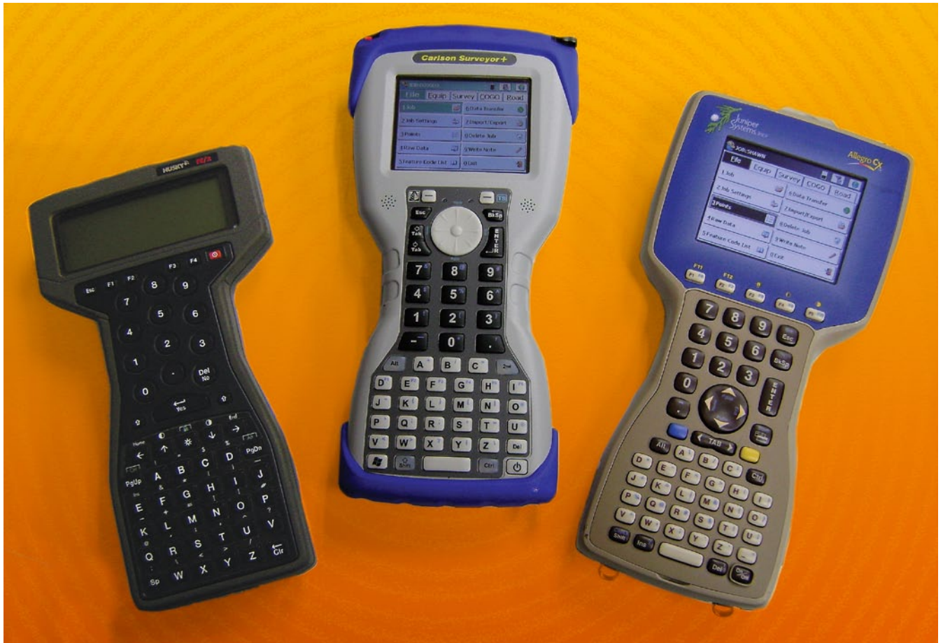
Pictured here are the Itronix Husky (now prehistoric by technology standards), the Carlson Surveyor, and Juniper System's Allegro. Even with its smoking fast processors and graphics, the Surveyor's durability is akin to that of the old Husky.
