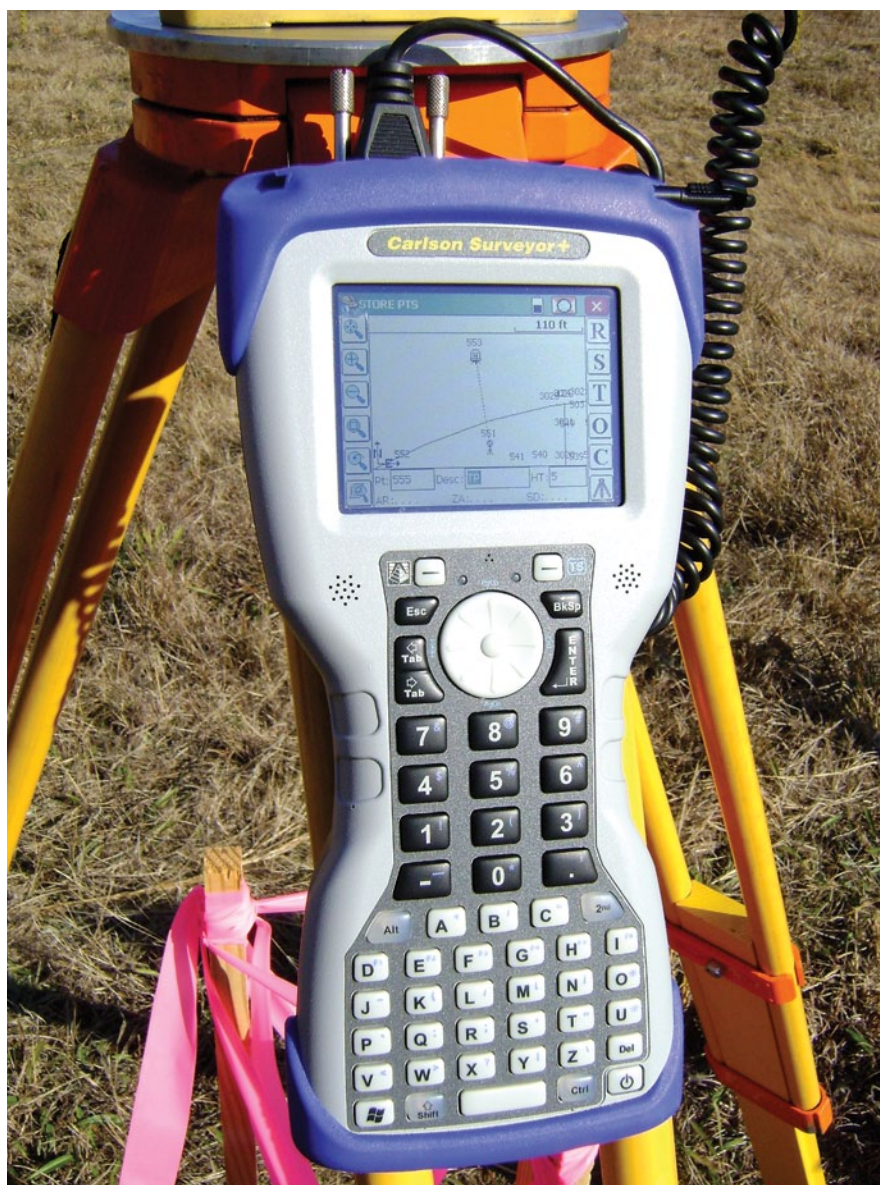
The Carlson Surveyor is capable of driving most current robot or RTK systems as well as conventional total stations. The built-in tripod hook on the back is especially convenient.
