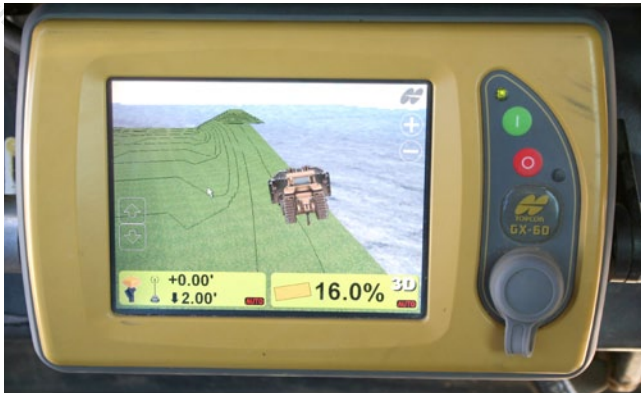
Topcon's GX-60 control box is a fully-functioning Windows computer that provides real-time grade information and control.
